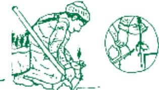
4. Slide your hand down the handle to the bracket. Pull blade up and back. Use the blade to scrape loose dirt out of the hole.
