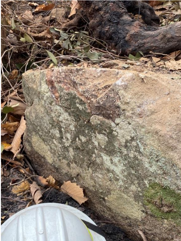
Photo #6 – View of “the rock” that cracked and caused the dozer to roll.
