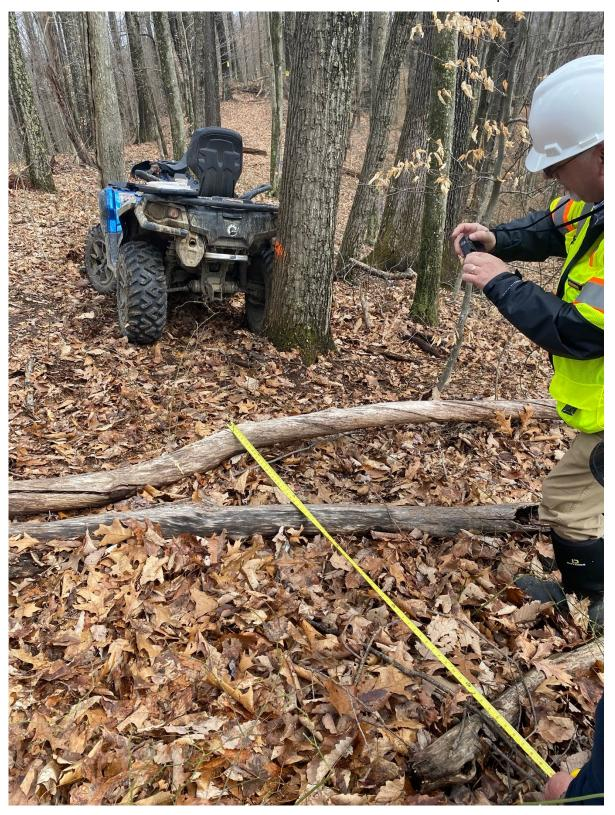
**4.** View of the ATV against the tree that it is believed to have partially climbed with the right front wheel. This is what is believed to have caused the ATV to overturn.
