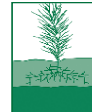
Trencher set too shallow.
