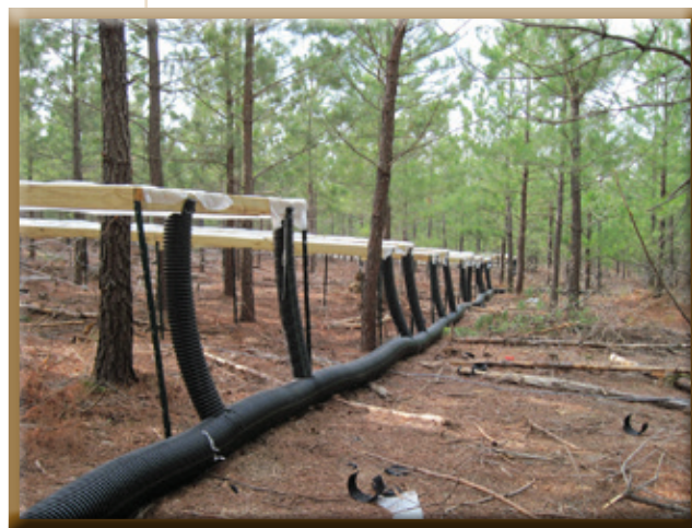
Rainfall exclusion devices on the PineMap project location at Appomattox-Buckingham State Forest studying the responses of loblolly pine to simulated drought and fertilizer additions.
