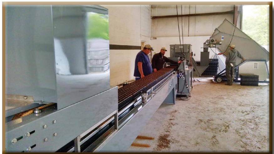
Mechanized Production Line for Containerized Seeding
